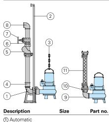
coupling system with mating flange, base elbow
